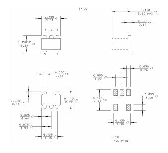
Dimensions are inches (millimeters) ±0.015 (0.38) unless otherwise specified.
